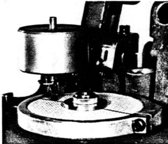
FIGURE 3—ATTACHMENT OF SCUFFING TEST FIXTURE TO ABRADER
